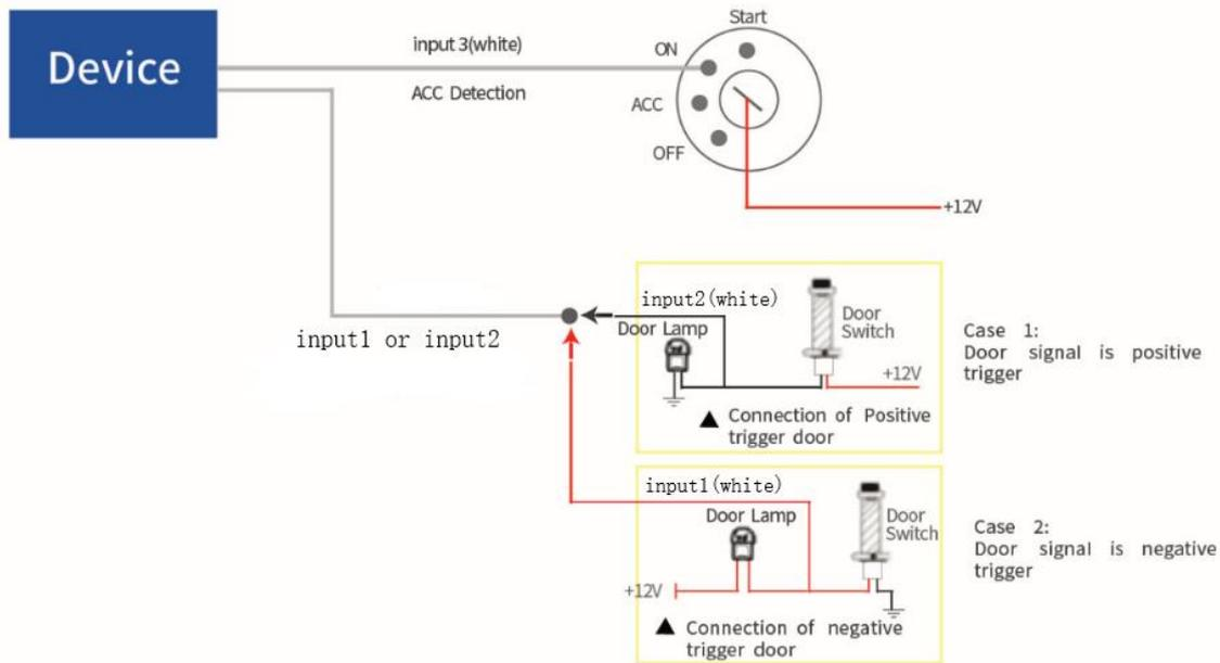
Input1 (VIL) can also be connected to PIN switch to detect the status of hood:
